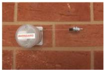
Fig.3. Digital tools for automatic crack monitoring – electronic data loggers (hoto by J. Gruntmanis): Resolution: 0.003 mm; Range: 80 mm; Linearity: 0.07 % throughout the range; Temperature sensor: -20 till + 80 °C; Resolution: 1 °C; Data capacity: 31926 readings; Power: CR2023 battery; Working temperature: -10 till + 60 °C
