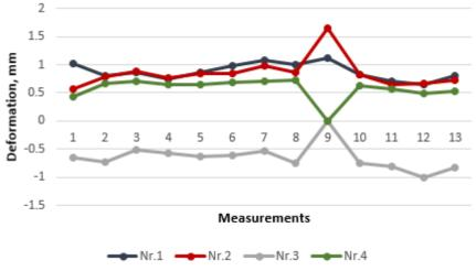
Fig. 8. Brick masonry deformation measurements
