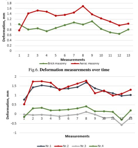
Fig. 7. Aeroc (aerated concrete block) masonry deformation measurements
