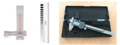
Fig. 2. Ruler sliding planes, crack width rulers and digital gauge (photo by J.Gruntmanis)
